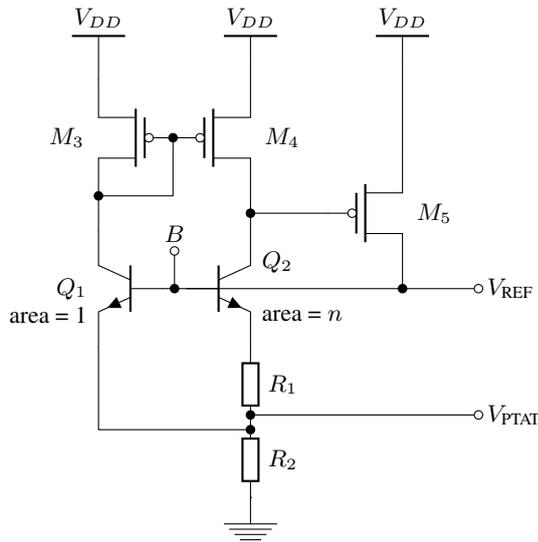
Fig. 1. Brokaw bandgap reference circuit. For simplicity, the start-up circuit has been omitted.
