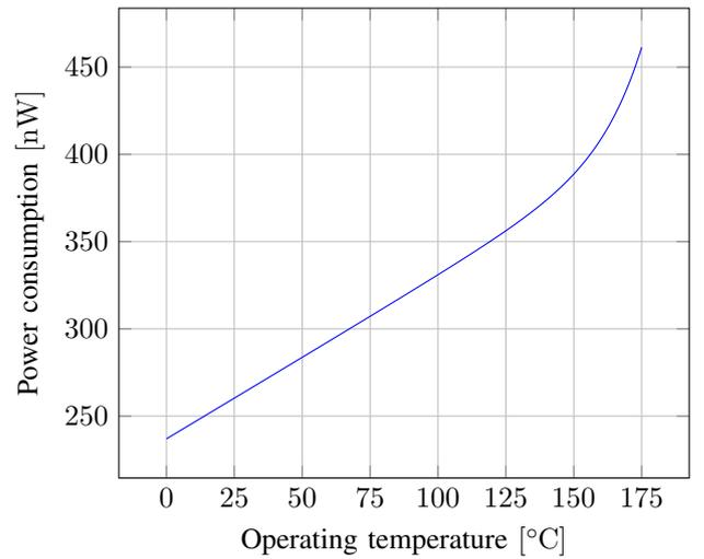
Fig. 5. Simulation result of the power consumption as a function of operating temperature for a Brokaw bandgap reference (Fig. 1) with compensation circuit (Fig. 2). The circuit was operated with a power supply of 2 V.
