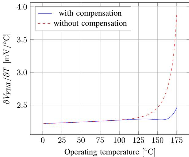
Fig. 4. Simulation result of the temperature sensitivity of the PTAT voltage,  $\partial V_{PTAT}/\partial T$ , as a function of operating temperature for a Brokaw bandgap reference (Fig. 1) with and without compensation circuit (Fig. 2).
