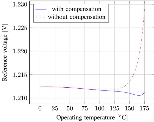
Fig. 3. Simulation result of the reference voltage,  $V_{REF}$ , as a function of operating temperature for a Brokaw bandgap reference (Fig. 1) with and without compensation circuit (Fig. 2).
