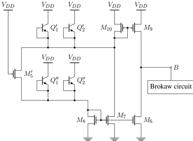
Fig. 2. Compensation circuit connected to the Brokaw bandgap circuit from Fig. 1. The prim/bis notation denotes devices identical to similarly named devices from the Brokaw bandgap circuit depicted in Fig. 1. Figure corrected after publication.
